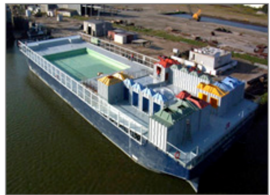
Jonathan Kirschenfeld's floating pool is made from a hollowed-out cargo barge. (Jonathan Kirschenfeld)
